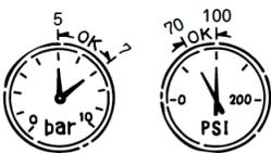
The tool is designed to operate within an air pressure range of 70 psi to 100 psi (5 to 7 bar). The pressure should be adjusted to the type of the work being fastened. The tool shall never be operated when the operating pressure exceeds 120 psi. (8.3 bar).
